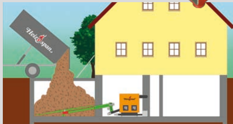
Underground storage for simple filling with agricultural equipment.
