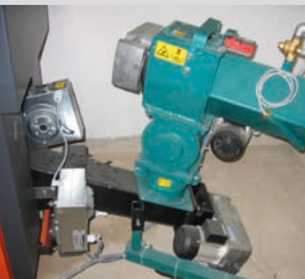
4 chamber rotary valve with counter blade.
