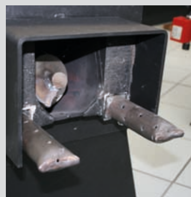
Stoker with primary air ducts.
