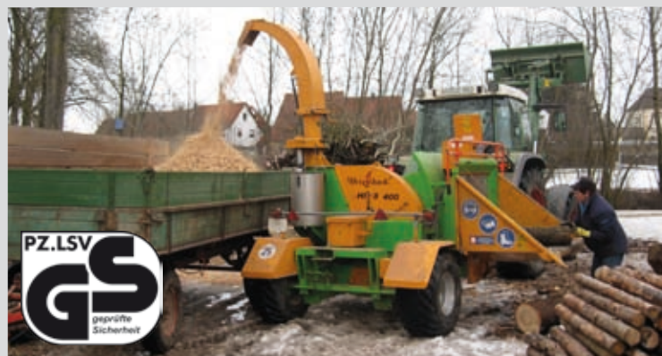
Heizohack hand-feed chipper for 30-40 cm diameter trunk.
