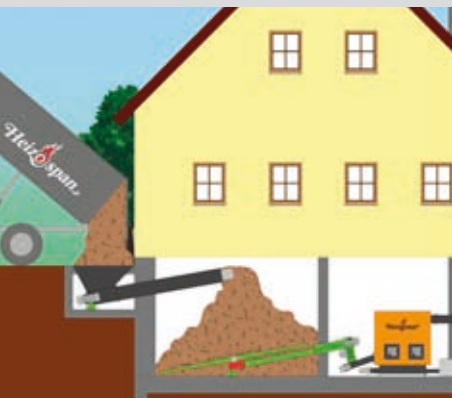
Inclined storage auger for internal fuel storage.
