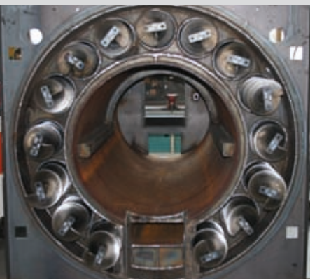
Generous heat exchanger with cleaning auger.
